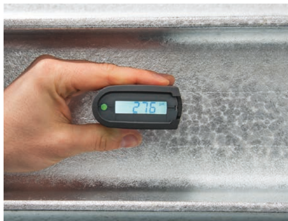
An LED shows immediately whether the value is within tolerance
