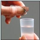
1. Drop one ExTab<sup>®</sup> reagent tablet into 20mL sample solution using cup provided.
