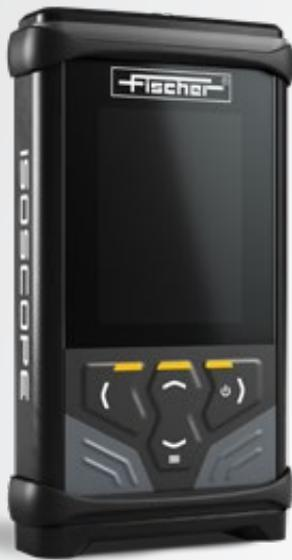
Measuring electrically insulated coatings on non-magnetized, electrically conductive metals
