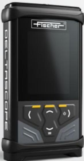
Measuring non-magnetized coatings on magnetized base materials
