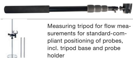
Measuring tripod for flow measurements for standard-compliant positioning of probes, incl. tripod base and probe holder
