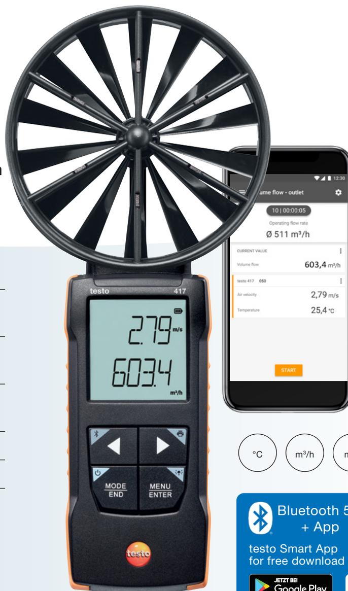
The compact vane anemometer testo 417 was developed to make it as easy as possible for you to take measurements on air inlets and outlets of **air conditioning and ventilation systems**. The integrated 100 mm vane quickly ensures precise results. Time and point average values as well as the volume flow are automatically calculated in the instrument and shown on the display.
